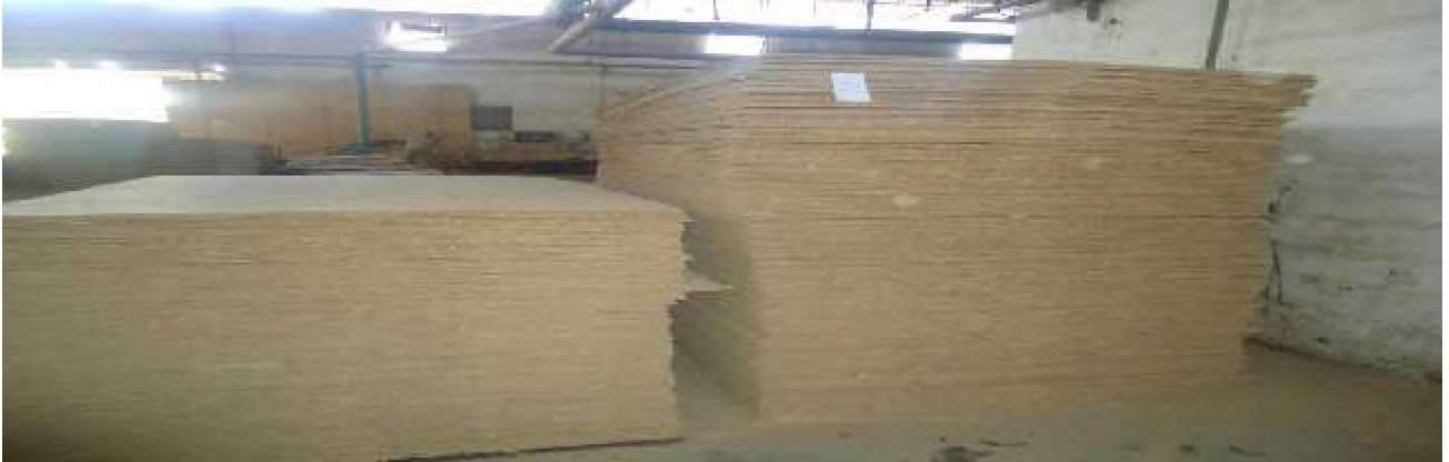
Figure 4.4 Chip wood board ready for sanding & cross cutting Source: - Picture taken during survey 2014/2015
