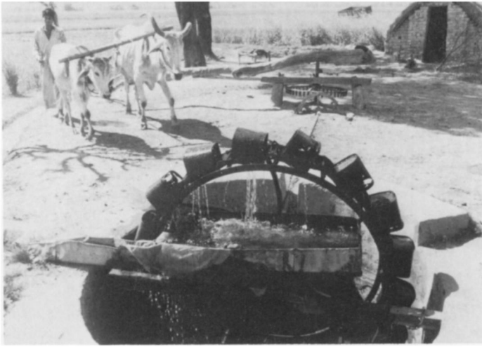
Figure 3. In the Indian village of Akbarpur-Barota, water to irrigate the fields is pumped by a Persian Wheel, powered by bullocks. Photo: Earthscan/Mark Edwards.
