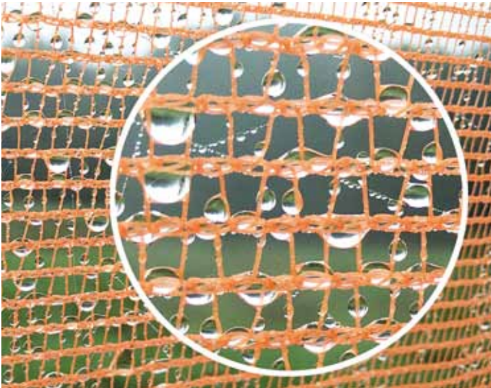
The mesh materials of fog collectors often mimic properties found in nature (from insects and plants) to maximise the amount of water collected. Photo credit: Warka Water http://www.warkawater.org/
