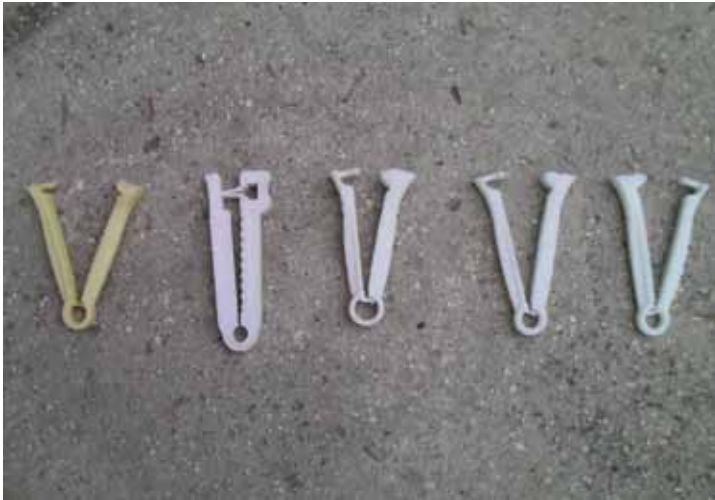
3D-printed umbilical clamps. Photo credit: Field Ready
