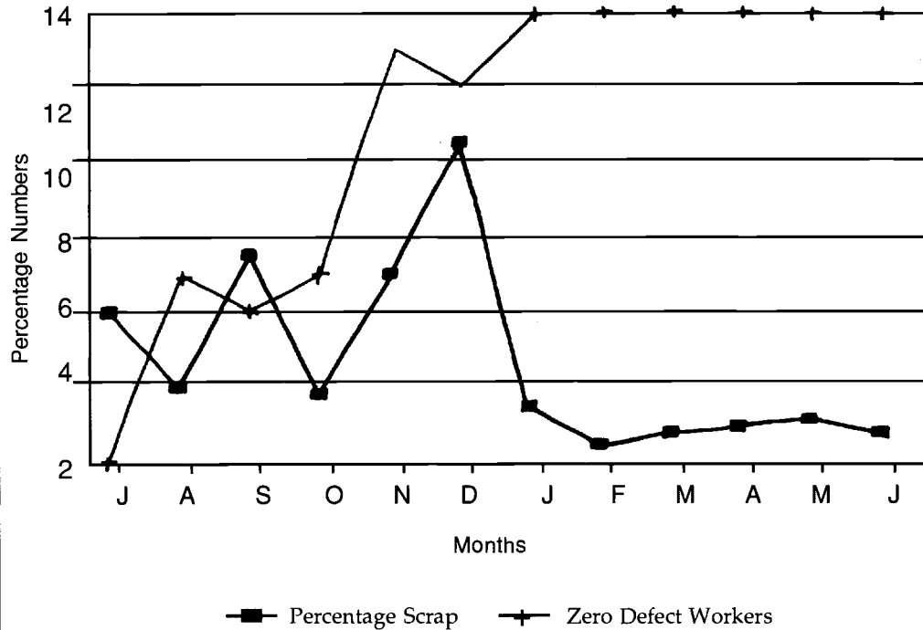
Figure 4: Crompton Greaves Ltd, Scrap and Zero Defect Operators at Ahmednagar Plant
