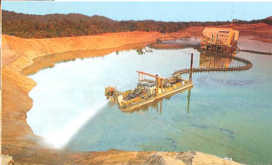
RBM uses a unique dredge mining process to remove valuable minerals from the sand dunes.
