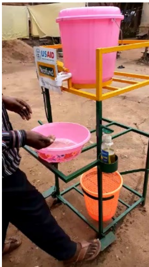
Figure 19: pedal-operated handwashing station. Credit: Tearfund DRC
