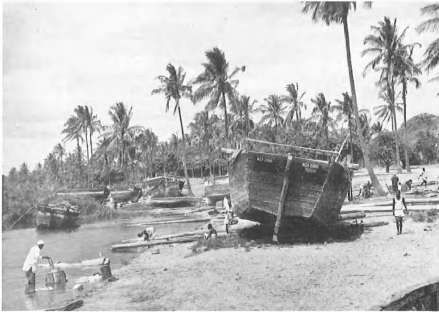
6 The dhow beach, Kirumba, Mwanza, Tanganyika. This beach, one and a half miles along the shore north of Mwanza, is the repairing centre for many of the Speke Gulf dhows. New dhows are also built here. The photograph shows beached dhows being repaired, a derelict dhow half submerged and the tall masts of eucalyptus wood lying on the sand. The coconut palms which give much of its charm to this beach are almost certainly relics of the Arabs who came from Lamu to build the dhows.
