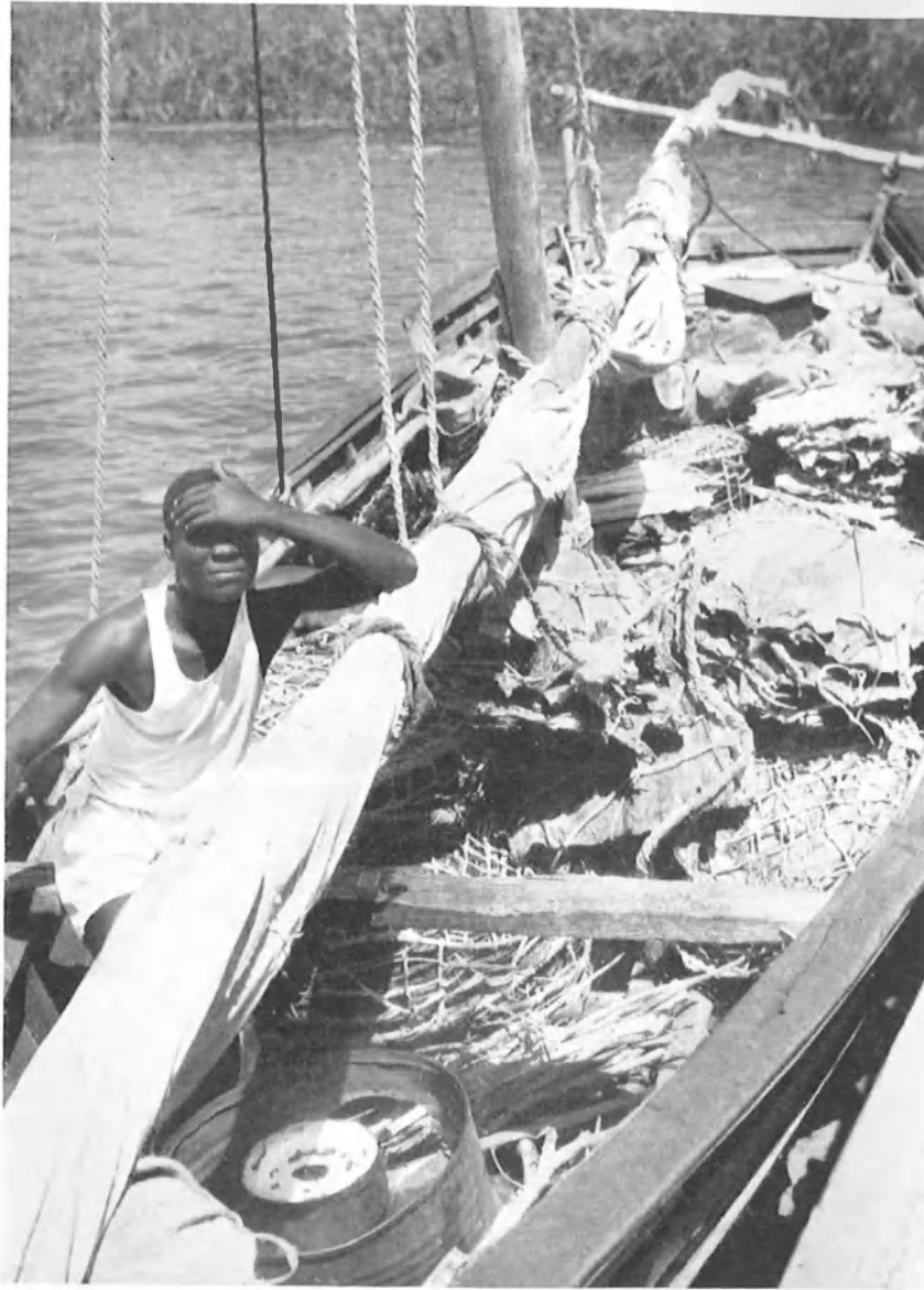
1 Fishing karua, Asembo Bay, Central Nyanza Kenya Colony. This small dhow is loaded with dried "ngege" and lung-fish brought from the Speke Gulf and Baumann Gulf. Note the lack of any accommodation for the crew and the typical galley, an old tin can filled with earth. The round wheel-shaped baskets containing the dried ngege are to be seen as well as the more shapeless bundles of dried lung-fish.
