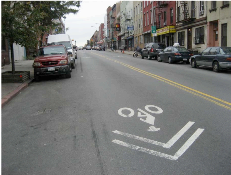
Figure 30: Where there is not enough room or cycling volume for a full bike lane, sharrows are used to indicate shared-use lanes, such as here on Greenpoint Avenue in Greenpoint, Brooklyn. (Source: Lewis Thorwaldson)
