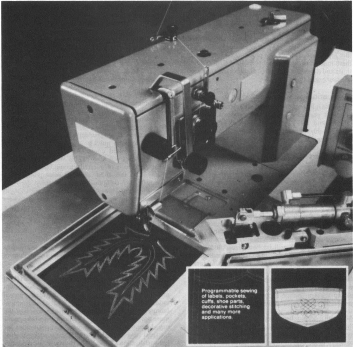
Microprocessor controlled sewing machine.
